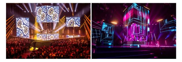
Also used on the show were 12 Platinum HFX, a mid-sized spot/ beam/wash moving head with the same intelligent optical system as the award-winning Platinum FLX. The FLX and HFX were positioned on two vertical trusses each side of the stage – 12 total on each side – with the FLX working from the outer truss. The hybrid modes of both fixtures were used throughout the show from backlight washes of color to big beam barrages to big gobo looks.
