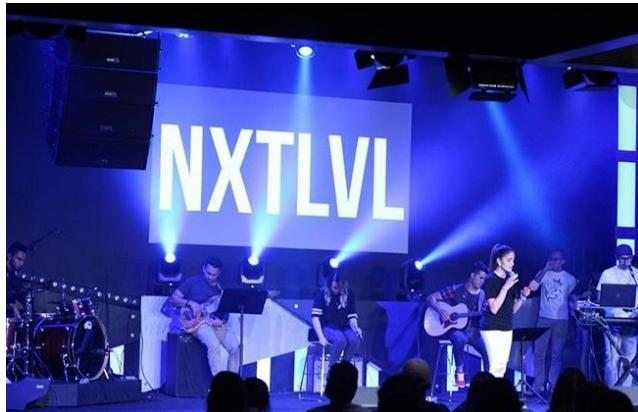
The lighting package in the youth auditorium, a large building that can seat up to 1,800 people, is used to light the auditorium stage and consists of 12 SixPar 100™ LED PAR lights, 6 Lumina Strip™ LED battens, 4 TVL 1000™ white light LED array panels, 4 Rayzor Q12 Zoom™ LED moving heads, and 6 Platinum Beam 5R Extreme beam lights. An Antari F-1 Fazer™ is used for atmospheric fog and haze effects.
