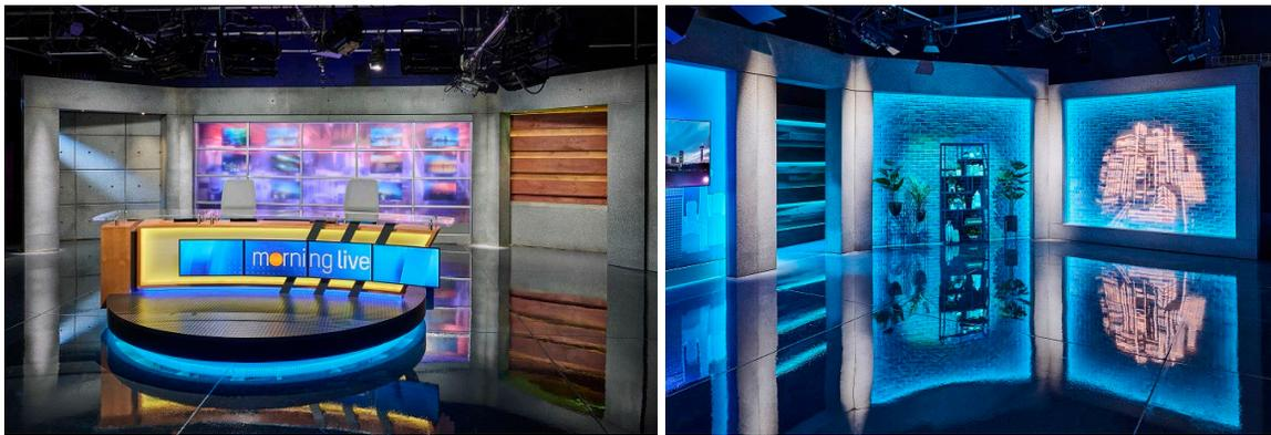
In addition, the team utilized [SixBar 1000™](#) battens to furnish accent lighting around the primary area of the set located behind the two anchors. McCormack emphasized the significance of these battens as they have the flexibility to change color and are incredibly versatile. Also included in the install and used for data distribution are NETRON [RDM 6XL™](#) DMX/RDM splitters from Obsidian Control Systems.
