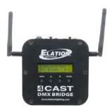
The Elation eCast will work with any Art-Net or sACN node but must first be connected to at least one 4Cast DMX Bridge to unlock the outputs. Audio trigger and MIDI support is also included.
