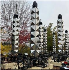
Another of the new colorful light features added in 2022 is Meadow Lake Magic. Here, Lightswitch conceived floating pontoon towers that ebb and flow as the water moves. Made up of vertical sections of truss clad in mirror panels and lit with Elation IP-rated <u>Paladin</u> floodlights, atop each pontoon sat a Proteus <u>Excalibur</u> beam light.
