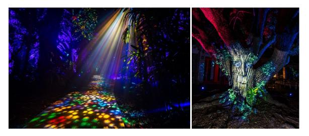
Populating several areas of the attraction with gobo breakups or custom gobos of whimsical forest characters were WW Profile IP warm-white ellipsoidal spots. The 130W ellipsoidals with framing shutters also served other purposes, for example lighting the tree canopy and illuminating the pathway so guests could more easily navigate through the experience.
