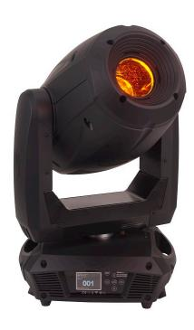
Using a high-performance 180W LED engine that gives a level of power comparable to a 575W discharge lamp, the fixture's flexible 4-blade rotating framing system allows the beam to be shaped and angled as required for precise highlighting of set pieces and performers, or can be used to create outstanding projection or midair effects.
