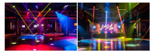
Above the dance floor is a rig of 10 Platinum Spot LED Pro II<sup>™</sup> moving heads, 8 Rayzor Q7<sup>™</sup> LED moving heads, and 8 Rayzor Beam 2Rs<sup>™</sup>, small and fast color- and gobo-changing moving heads
