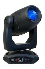
The Satura Spot CMY's 320W LED engine delivers 11,700 lumens of power for an output across all colors that is comparable to 575W and even 700W discharge fixtures. It projects the flat field of light that designers favor with sharp zoom optics that emit a powerful, well-defined beam. For flexible beam angle adjustments, the Satura Spot CMY houses a 14-36 degree zoom with a uniform field of light that is maintained throughout the zoom range.
