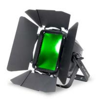
A 90° x 113° elliptical beam angle gives a broad, asymmetrical wash of light while 8-leaf adjustable barn doors (included) allow for customized shaping of the beam for more precise illumination and less light spill. The fixture comes outfitted with 64 internal color macros and strobe effects and selectable dimming curve effects add to its design possibilities.
