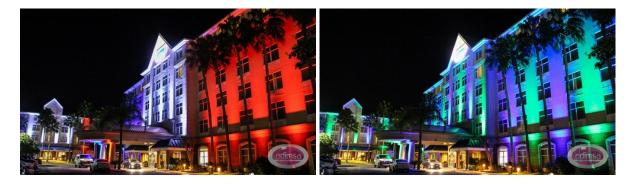
The fully weatherproof SixPar lights house 6-color LED multi-chips that allow for an expanded palette of colors which are used to highlight and enhance the front of the hotel in a variety of decorative shades. Installed at ground level, the first floor cornice and in front of columns at the hotel's motor lobby, the SixPar 200's twelve 12W LEDs and 15° beam angle allow for full coverage illumination along the entire height of the hotel's façade as well as uniform transitions between fixtures.
